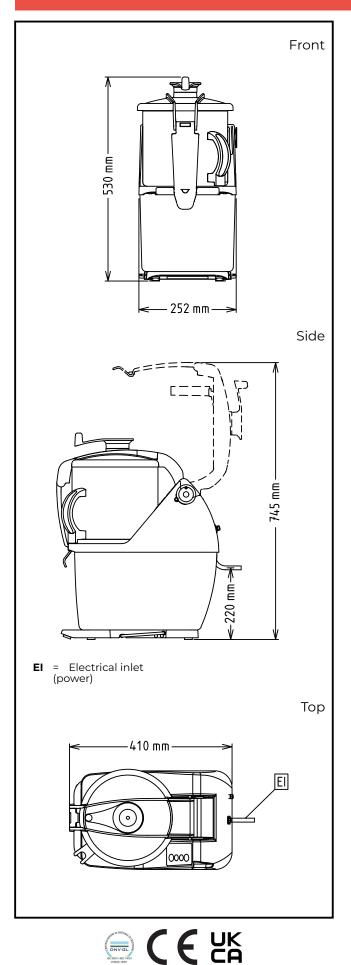
Electric Supply voltage: 200-240 V/1N ph/50/60 Hz Capacity: Performance (up to): 550 kg/hour 7 litres Capacity: Key Information: External dimensions, Width: 252 mm External dimensions, 485 mm Depth: External dimensions, 505 mm Height: **Shipping weight:** ISO 9001; ISO 14001 kg
